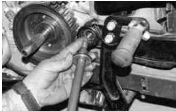
**Fig. 4 Use special seal supplied with kit, countersunk side facing head of pivot bolt. Replace shaft with bolt on drive side of bike. Install spacer supplied using stock o-ring, and install castle nut.**
